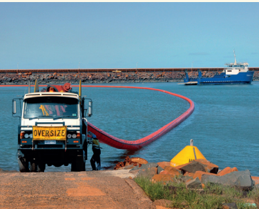
Deployed from Land 300 metres fully inflated in 5 minutes
